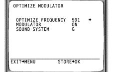
Tune in the TV set to the new modulator frequency (channel 21 - 69) shown in the video recorder display.
